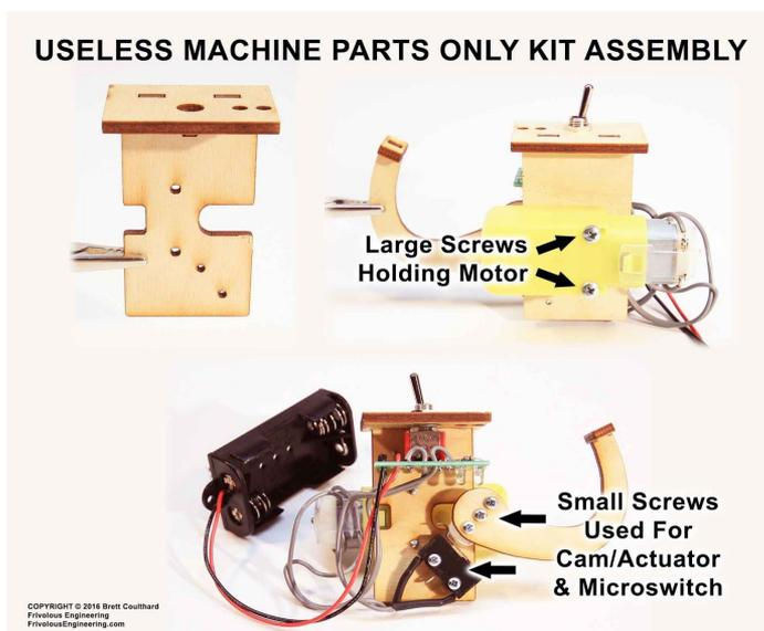
Attach the Motor to the Motor-Mount Bracket using the two large screws. They go from the motor side and screw into the Motor-Mount as shown.
